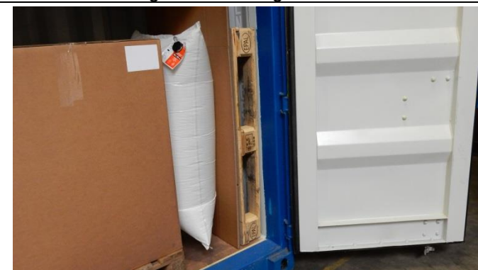
If void is too wide, add buffer material
